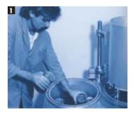
**1.** 5 flasks are placed in the mixer and the stirring unit is swivelled over them.
